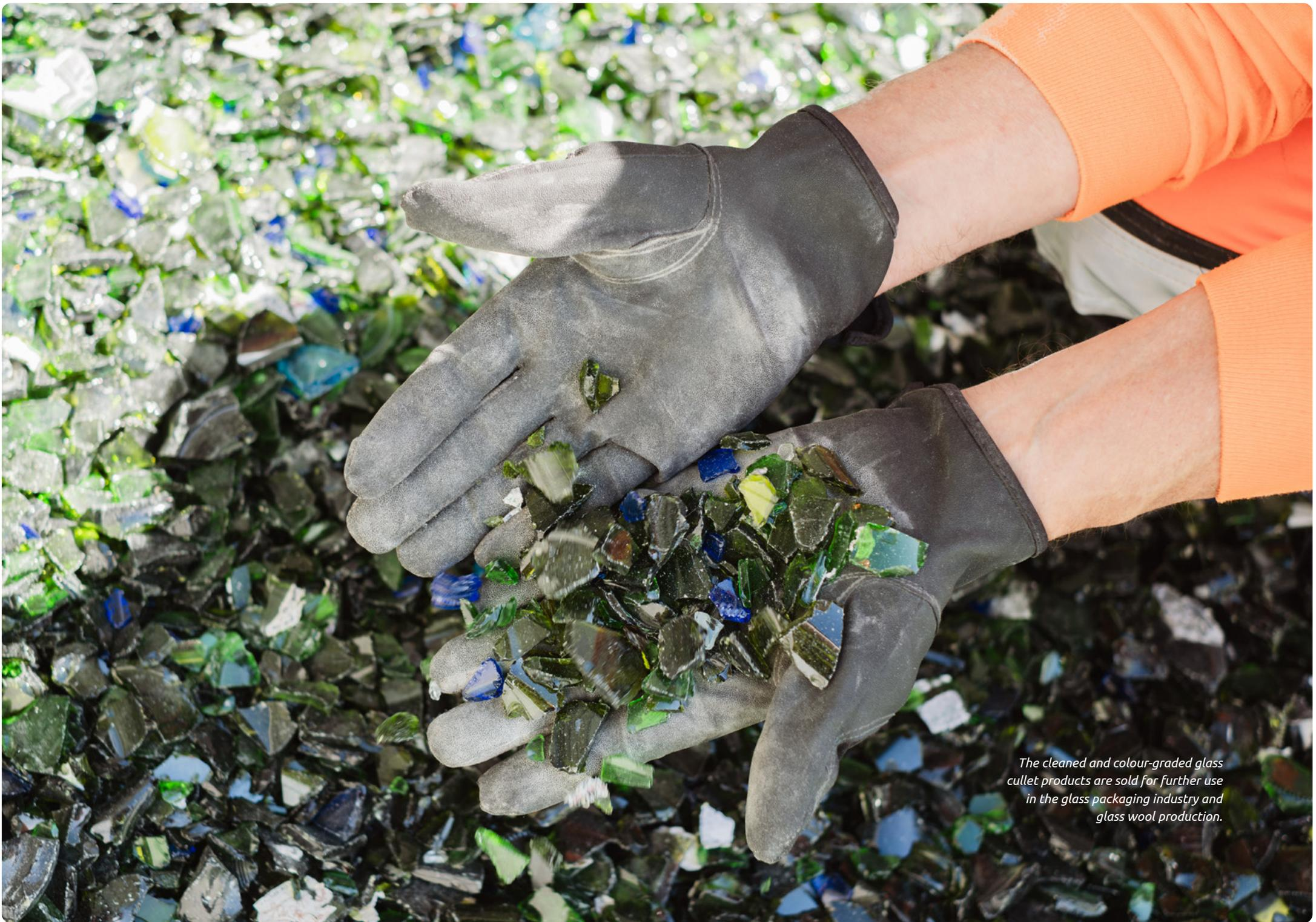
*The cleaned and colour-graded glass cullet products are sold for further use in the glass packaging industry and glass wool production.*
